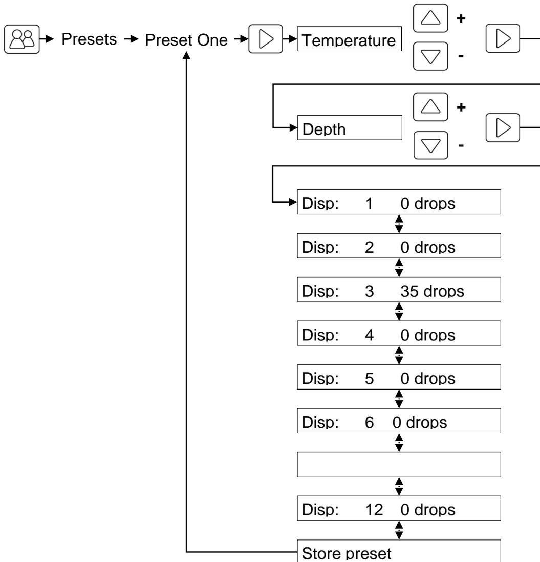
To change the values of a preset press and using the / buttons select the presets you wish to alter. Button takes you to the preset variables one by one starting with Temperature, followed by depth, etc. To increase/decrease the value of a variable use / . The button takes you a step back.
